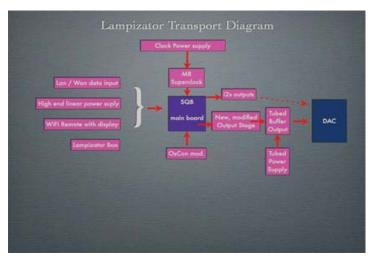
As you can see the mainboard got a new power supply, MR superclock, LAN/WAN input data input, and modified output stage with tubed buffer. Yes, the latter component might surprise you most but according to Mr. Fikus it simply sounds better with tubes than without them – he sells the product so he wants it to sound best; no reason not to believe him.
